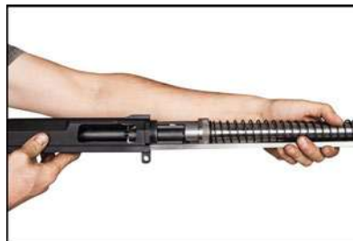
10) Separate the Barrel from the Upper Receiver
