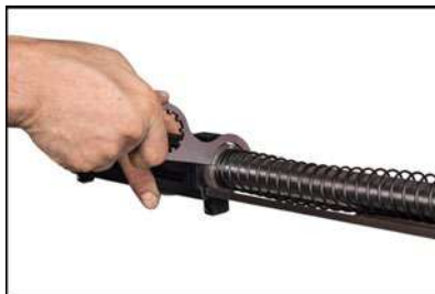
9) Take out the Barrel Assembly Nut by Turning Counterclockwise
